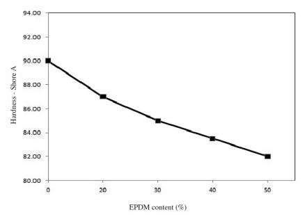
FIGURE 3. Effect of EPDM loading on hardness of PP/EPDM blend
