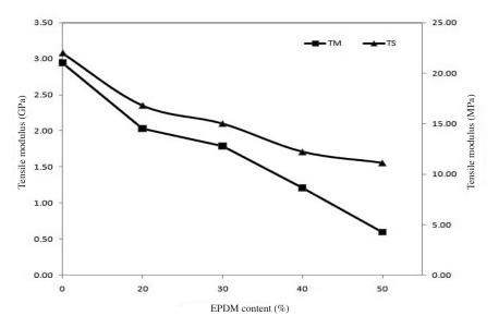
FIGURE 1. Effect of EPDM loading on tensile modulus and tensile strength of PP/EPDM blend
