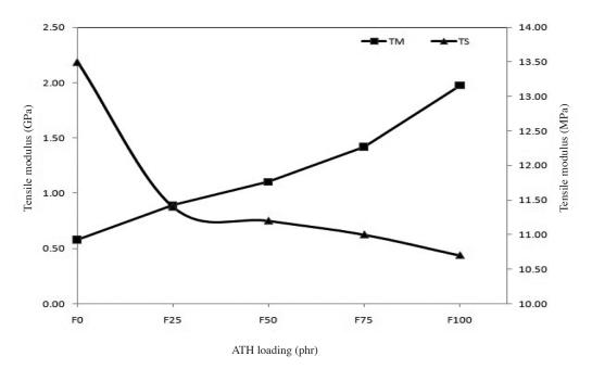
FIGURE 4. Effect of ATH loading on tensile modulus and tensile strength of PP/EPDM blend
