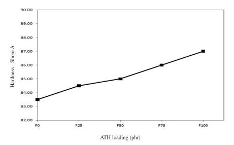
FIGURE 6. Effect of ATH loading on hardness of PP/EPDM blend
