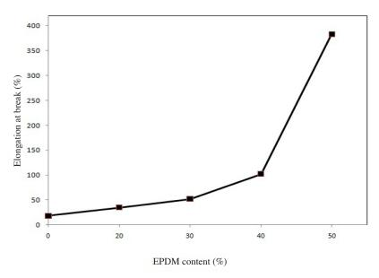
FIGURE 2. Effect of EPDM loading on elongation at break of PP/EPDM blend
